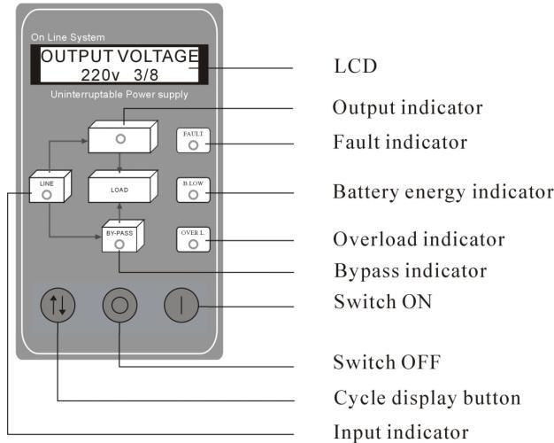
Figure 1. Symbol instruction of front panel indicator
