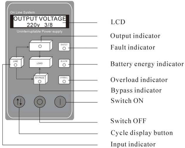
Figure 1. Symbol instruction of front panel indicator
