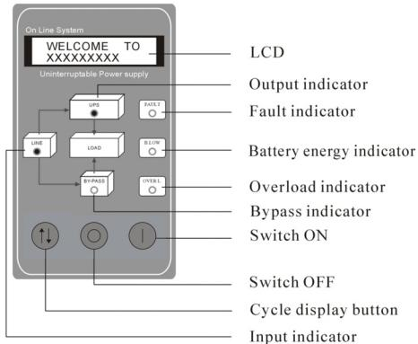
4. Shutdown input power of UPS, utility indicator light is off, the welcome information is displayed on LCD, and output is UPS inverter powered, as following drawing. UPS sounds every four seconds, which indicates UPS runs on battery mode at present. The sound will automatically stop 90s later. UPS will sound alarm every 1s again when battery power is to be exhausted.
